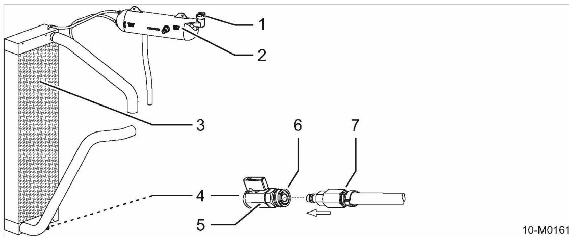
Fig. 48 Draining the coolant from the radiator
