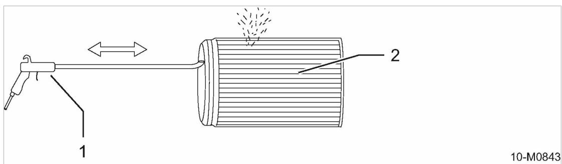
Fig. 70 Cleaning the filter element
