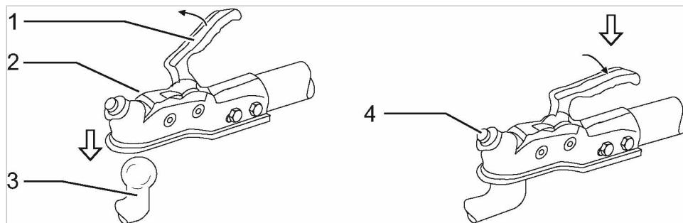
Fig. 83 Ball coupling (ALKO-EU)
