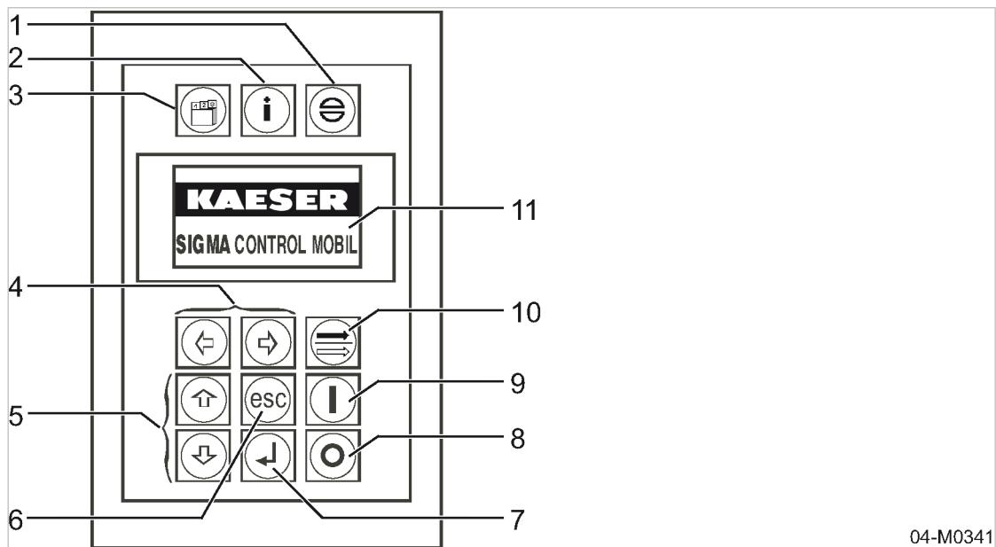
Fig. 7 Instrument panel keys and displays
