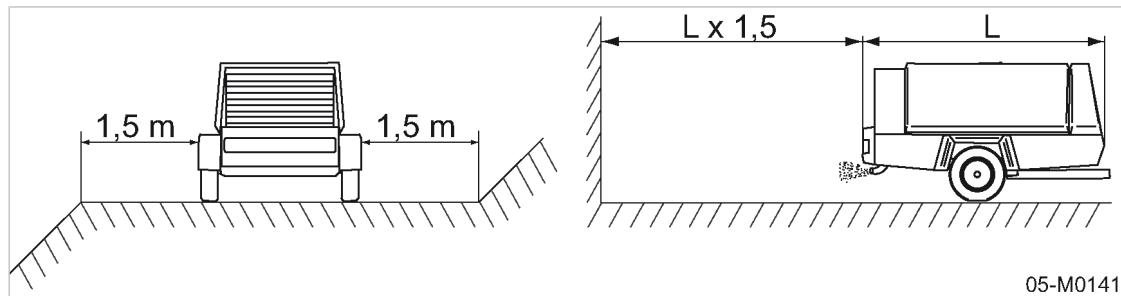
Fig. 23 Minimum distance from excavations/slopes and walls
