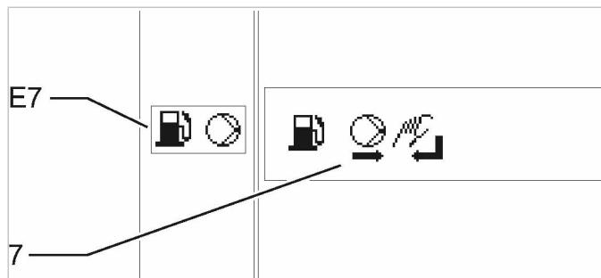
Fig. 46 External fuel pump switch-on symbol
