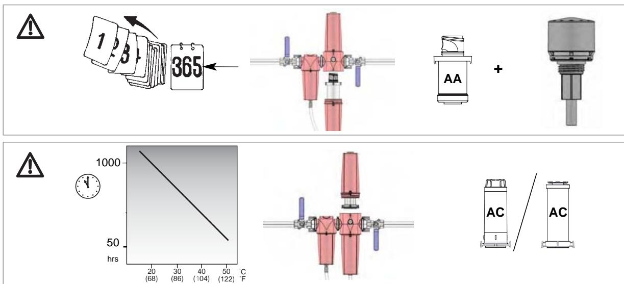
Models AC010□□□I - AC030□□□I are fitted with a bulk oil indicator. Both filter elements and indicator should be changed if indicator is blue in colour.
