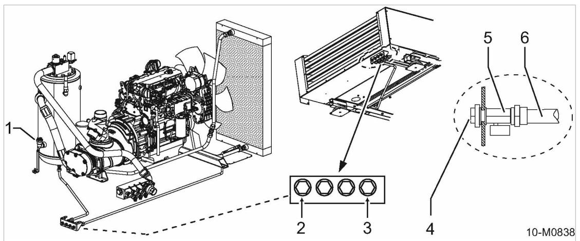
Fig. 65 Central compressor oil drainage
