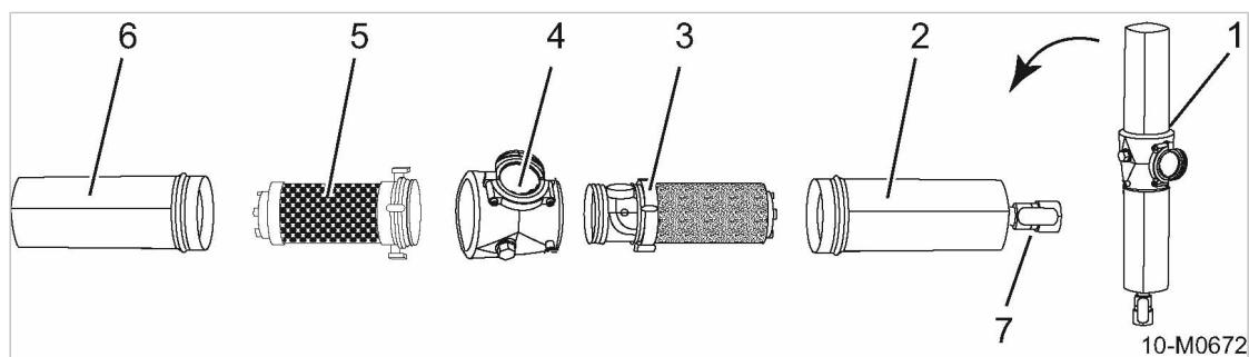
**Fig. 80 Breathing air filter maintenance**
