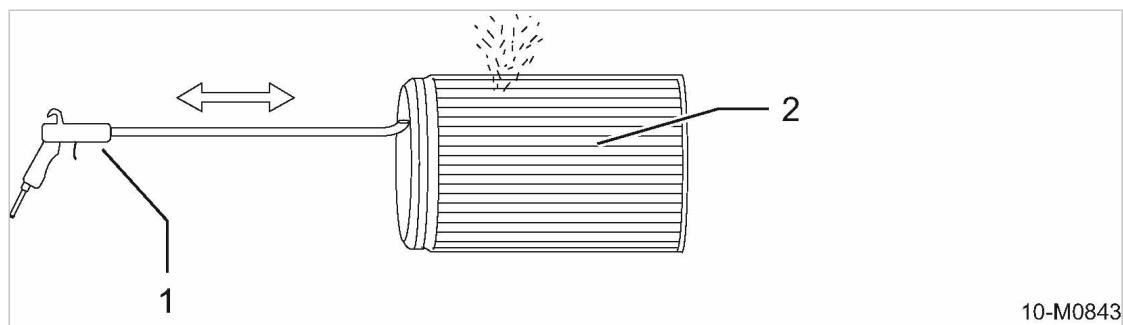
Fig. 51 Cleaning the filter element
