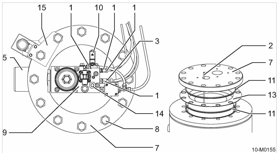
Fig. 68 Changing the oil separator cartridge
