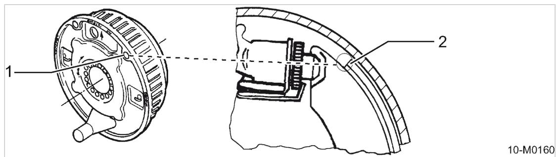
Fig. 76 Checking the brake lining thickness
