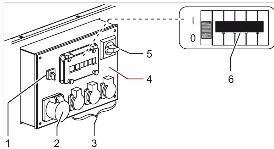
Fig. 21 Generator instrument panel - control box, 400 V, 3-phase
