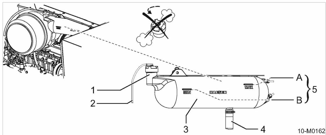
Fig. 47 Checking coolant level
