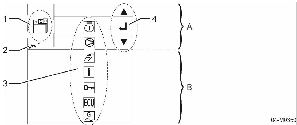
Fig. 11 Menu structure of the SIGMA CONTROL MOBIL
