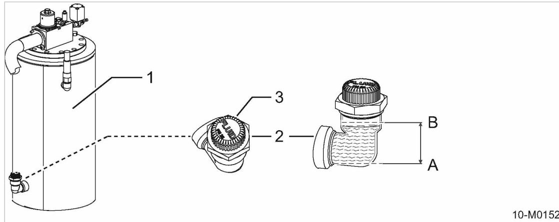
Fig. 63 Checking cooling oil level
