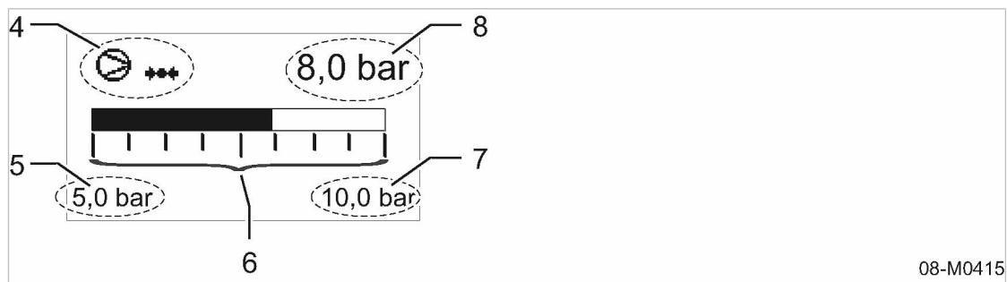
Fig. 44 Setting the output pressure
