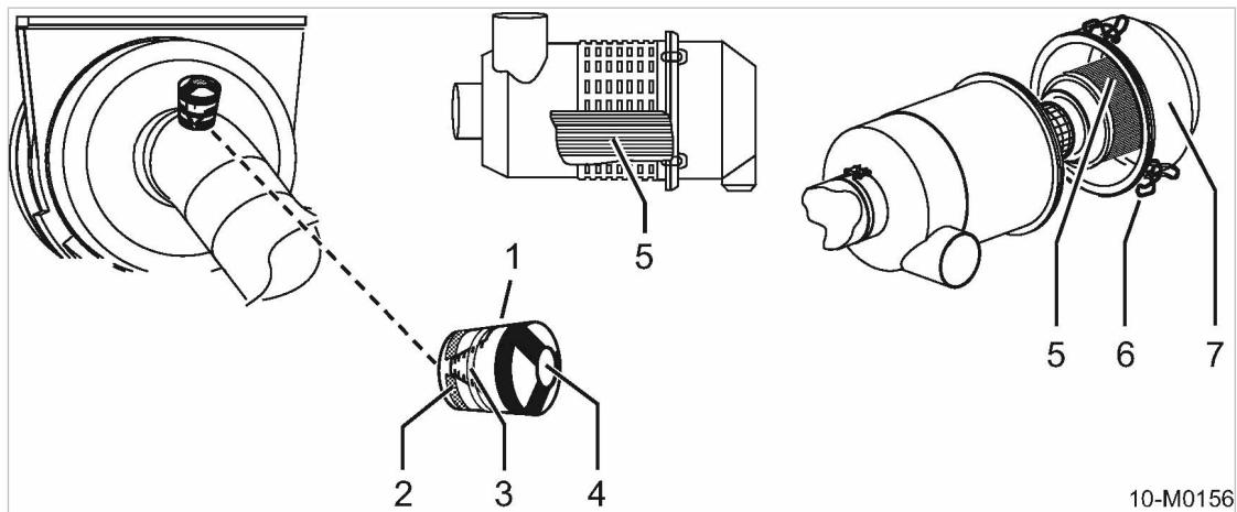
Fig. 69 Compressor air filter maintenance
