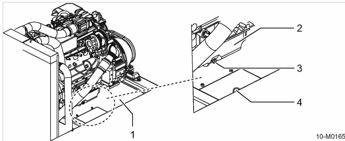
Fig. 58 Draining the engine oil
