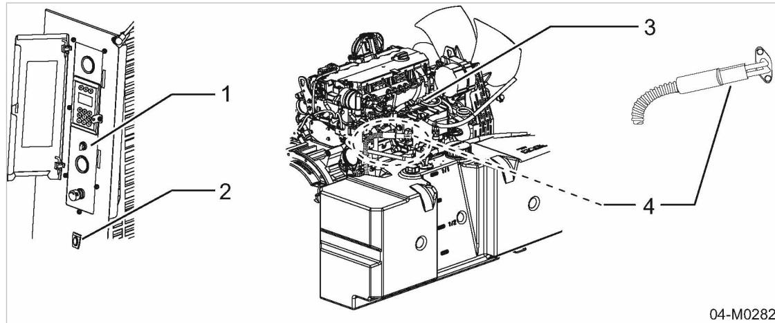
Fig. 20 Coolant pre-heating
