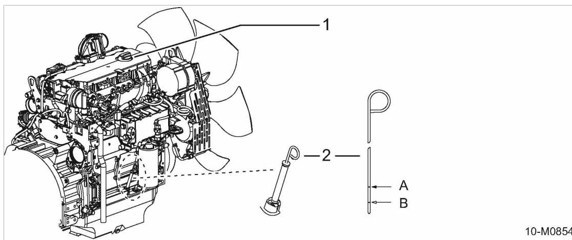
Fig. 57 Checking the engine oil level
